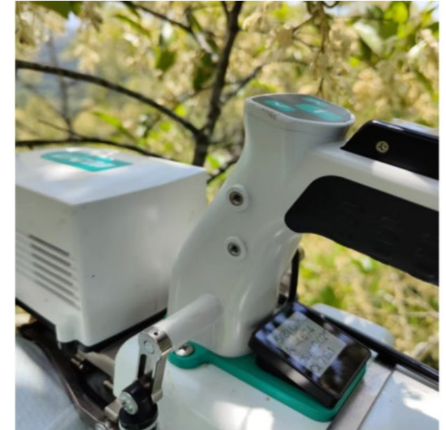
Portable photosynthesis system (Li-6800, Li-COR, Lincoln, NE, USA)
