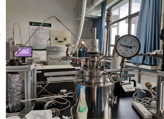
1: speed control; 2: temperature control; 3: heating control; 4: operation panel; 5: exhaust valve; 6: stirring motor; 7: heating jacket; 8: stirrer; 9: thermocouple; 10: pressure gauge; 11: intake valve; 12: booster pump; 13: compressed air; 14: CO 2 gas source
