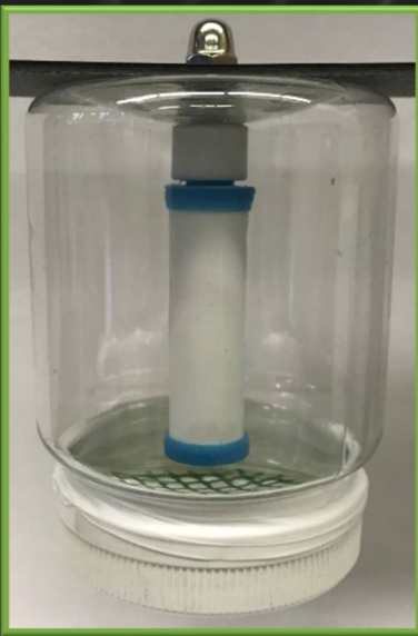
The final, assembled graphene foam PAS prototype
