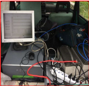
Picarro® G2201-i Analyzer : cavity ring-down spectroscopy for CO 2 and CH 4 CO 2 : from air concentration up to 2000 ppm CH 4 : High Precision (1.8 – 12 ppm) & High Range (up to 1000 ppm)
