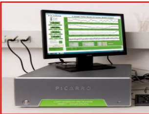
Picarro® G2201-i Analyzer : cavity ring-down spectroscopy for CO 2 and CH 4 CO 2 : from air concentration up to 2000 ppm CH 4 : High Precision (1.8 – 12 ppm) & High Range (up to 1000 ppm)
